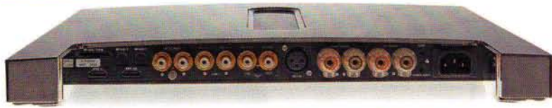
ABOVE: Devialet has equipped its amp with an HDMI v1.3 input and output, two Toslink optical digital inputs (up to 24-bit/192kHz) and a balanced AES/EBU digital input. The MM/MC phono and line input, two coaxial digital inputs/outputs (up to 24-bit/192kHz) may be configured to use any of the six visible RCA sockets.
